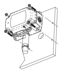
Fig. 5: Outside Humidity in a BAPI-Box (BB) Enclosure
