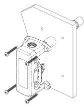
Fig. 3: Duct Humidity in a BAPI-Box 2 (BB2) Enclosure
