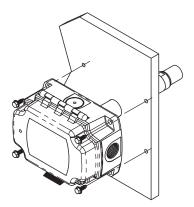
Fig. 2: Duct Humidity in a BAPI-Box (BB) Enclosure
