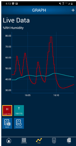
Fig. 10: Graph Screen showing two logs. The red humidity log is selected as the primary log so the scale values on the axes only apply to that graph.
