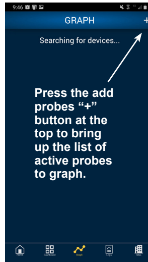
Fig. 11: Initial Graph Screen showing the add probes “+” button to add probes.
