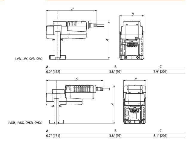
On/Off, Floating Point, Electrical Fail-Safe, Linear, 120 V
