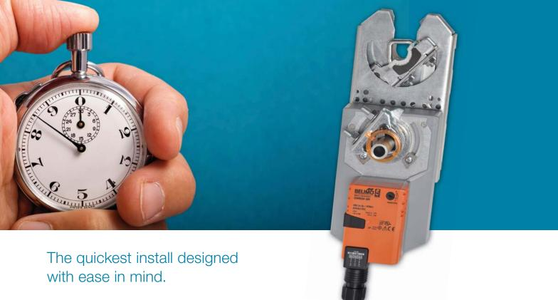
The ZG-JSL linkage is designed to facilitate the attachment of select Belimo actuators to a damper's jackshaft. The unique open ended design allows the linkage to clamp on to any part of a jackshaft measuring from 1/2" to 1.05" in diameter.
