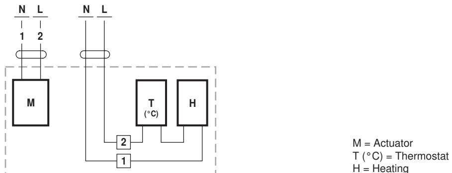
Examples of external wiring with actuator types ..XUP..N4
