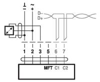
Connection with switching contact, e.g.  $\Delta p$  monitor
