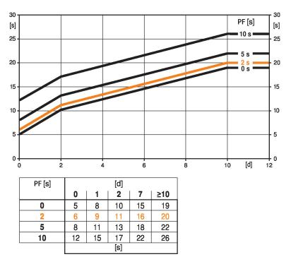
[d] = Power failure in days [s] = Pre-charging time in seconds PF[s] = Bridging time Calculation example: Given a power failure of 3 days and a bridging time (PF) set at 5 s, the actuator requires a pre-charging time of 14 s after the power has been reconnected (see graphic).
