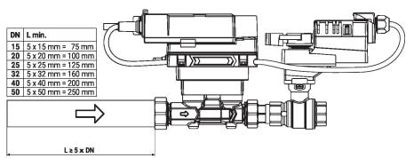
**Split installation** The valve-actuator combination may be mounted separately from the flow sensor. The direction of flow of both components must be observed.
