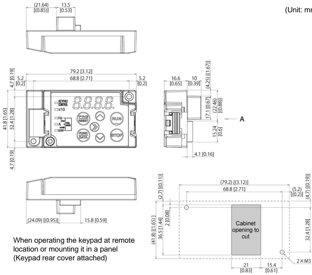
When operating the keypad at remote location or mounting it in a panel (Keypad rear cover attached)
